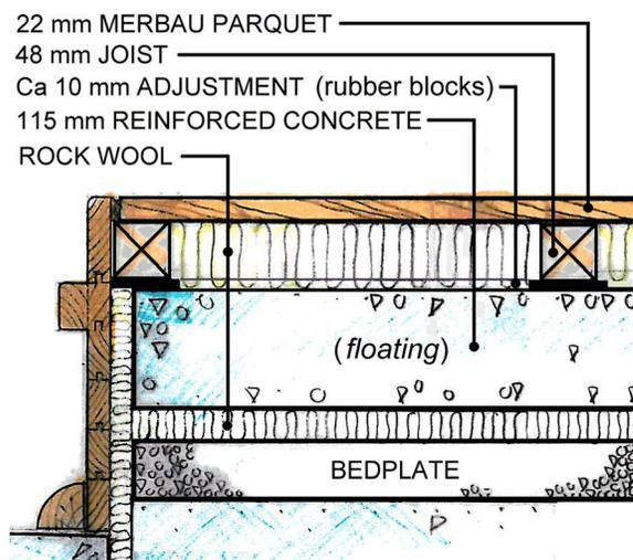
FIG. 1. (Color online) Stage-floor construction in LiH. The joists, only 30 cm apart, are resting on floating, reinforced concrete, with thin rubber blocks in between. (Drawing made available by courtesy of Arkitektgruppen Lille Frøen AS.)
